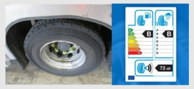
As such, B or C rated RR tyres (which are less robust than D or E rated tyres) ought to be acceptable for the application and would save significant fuel.
