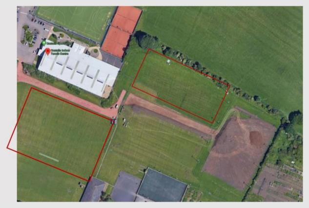
The distance between the nearest walls of the tennis Centre and university building is 78m and the majority of this would be soft dig. The additional distances between plant rooms must be considered.
